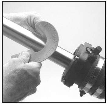
**14** Pull the red seal protector from the SureSeal. Separate the tabs to split the cone and remove it from the shaft.
