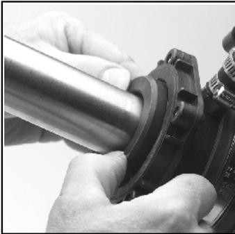
**6** Carefully slide the new lip seal down the shaft and into the chamfered opening in the front of the housing.
