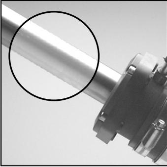
**1** Determine where the Spare Seal Carrier will be located on the shaft (minimally 1" from the SureSeal™) and be certain there are no keyways, nicks or corrosion in this area which could damage the lip seal.
