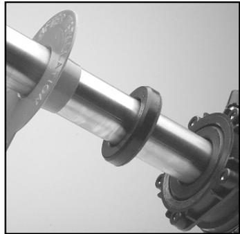
**5** Remove the red seal protector and confirm that each spare seal is facing the same direction as the lip seal in the SureSeal™ unit.
