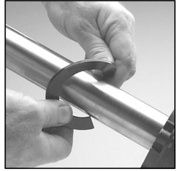
**7** Return the split retaining washer to the shaft in front of the lip seal.
