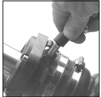
**15** Connect the STRONG® SureSeal™ to a pressurized water supply source (point in the engine's raw water cooling system) by attaching the water injection hose to the stainless steel fitting on the housing. If there is a second hose fitting on the SureSeal, it is used to complete a crossover feed between the port and starboard shaft seals. Complete crossover instructions are included with STRONG® Water Pick-Up Kits and should be followed closely.
