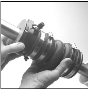
**10** Carefully slide the assembly (hose end first) onto the shaft so that the shaft passes through the red seal protector.
