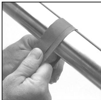
**7** Examine this area carefully. Be sure that it is free of pitting, nicks or surface imperfections which could cause leaking. Clean this area thoroughly. Polish the shaft using 300 grit wet/dry sandpaper or emery cloth working around the shaft. Fore and aft actions could put flats or grooves in the shaft. The assembly may be shifted forward slightly by adjusting the position of the hose on the stern tube at the time of installation.
