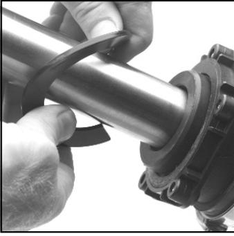
**4** Separate the split retaining washer and remove it from the shaft.
