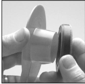
**3** Carefully press each spare seal onto the tapered protective cone -smooth side (with part number imprint) first.
