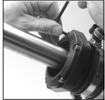
**9** Alternately tighten cap screws in a criss-cross pattern, driving the lip seal into the opening. Seal is seated properly when cap and housing touch.
