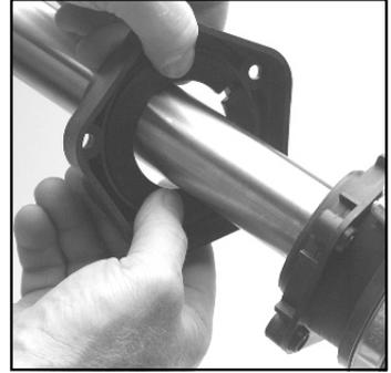
**8** Fit the split retaining washer into its recess inside the cap. Slide cap and washer until they touch the lip seal. Align holes and start cap screws.
