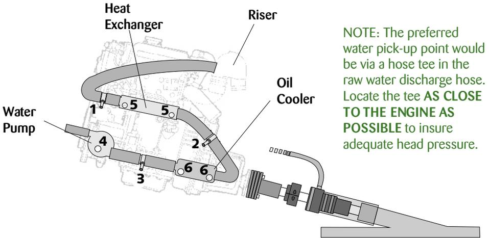
NOTE: The preferred water pick-up point would be via a hose tee in the raw water discharge hose. Locate the tee AS CLOSE TO THE ENGINE AS POSSIBLE to insure adequate head pressure.
