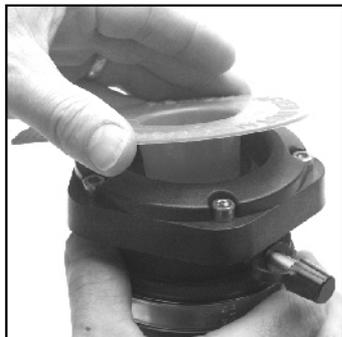
**8** Carefully press the red seal protector into the front of the SureSeal. Make certain it covers the "lip" portion of the seal.
