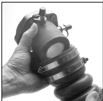
**5** Insert the end of the SureSeal unit into the articulated hose and push in as far as it will go.
