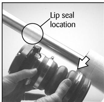
**6** Position the hose as shown next to the stern tube to determine approximately where the lip seal will ride on the shaft.
