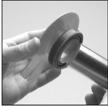
**4** Slide the protector and seal(s) onto the shaft as shown- seal side first.
