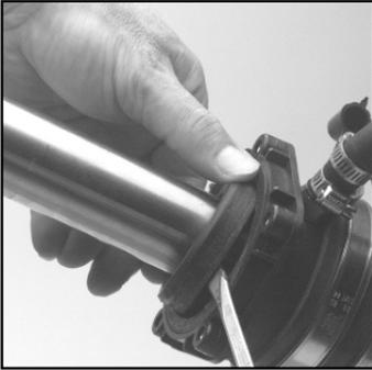
**5** Pry out the old lip seal with a screw driver working alternately on opposite sides. Cut old seal off shaft with diagonal pliers.
